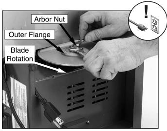
Figure 11. Removing the arbor nut.
